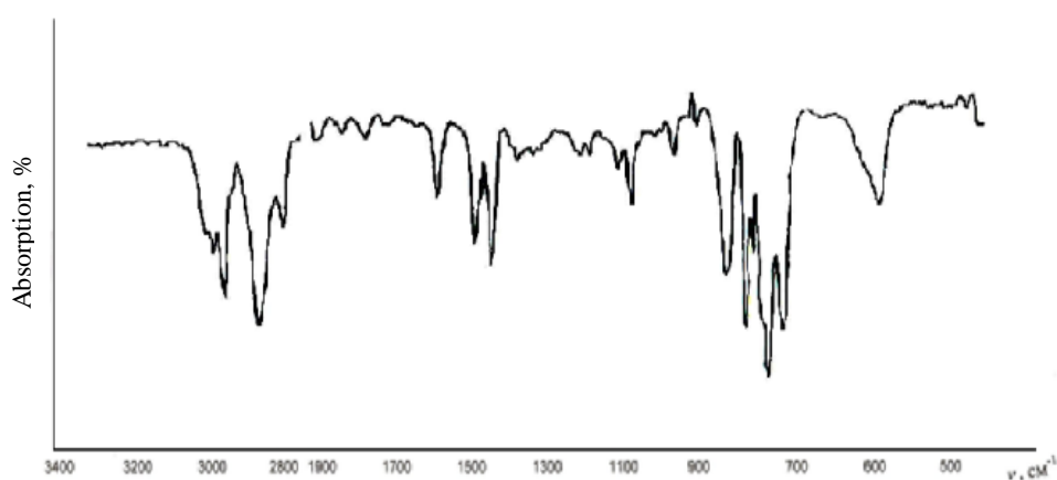
Figure 1. IR spectrum of sulfonic cation exchangers synthesized based on modified mixture OPS:PVC:filler. PVC content - 2% (wt.); filler 4% (wt.)
