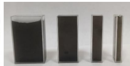
c) Suspencion based on MWCNT in cuvettes with different thicknesses
