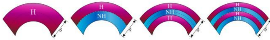
Figure 2. Sectional profile and material layering scheme of multilayered HTI cylindrical shells
