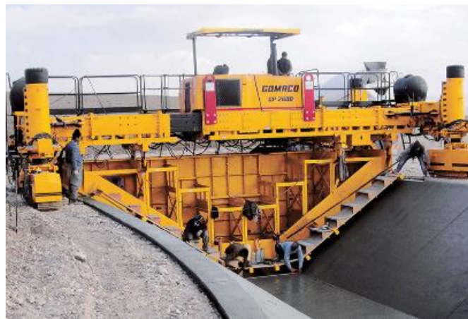
Figure 5. Concrete paver machine GP-2600 manufactured by GOMACO company
